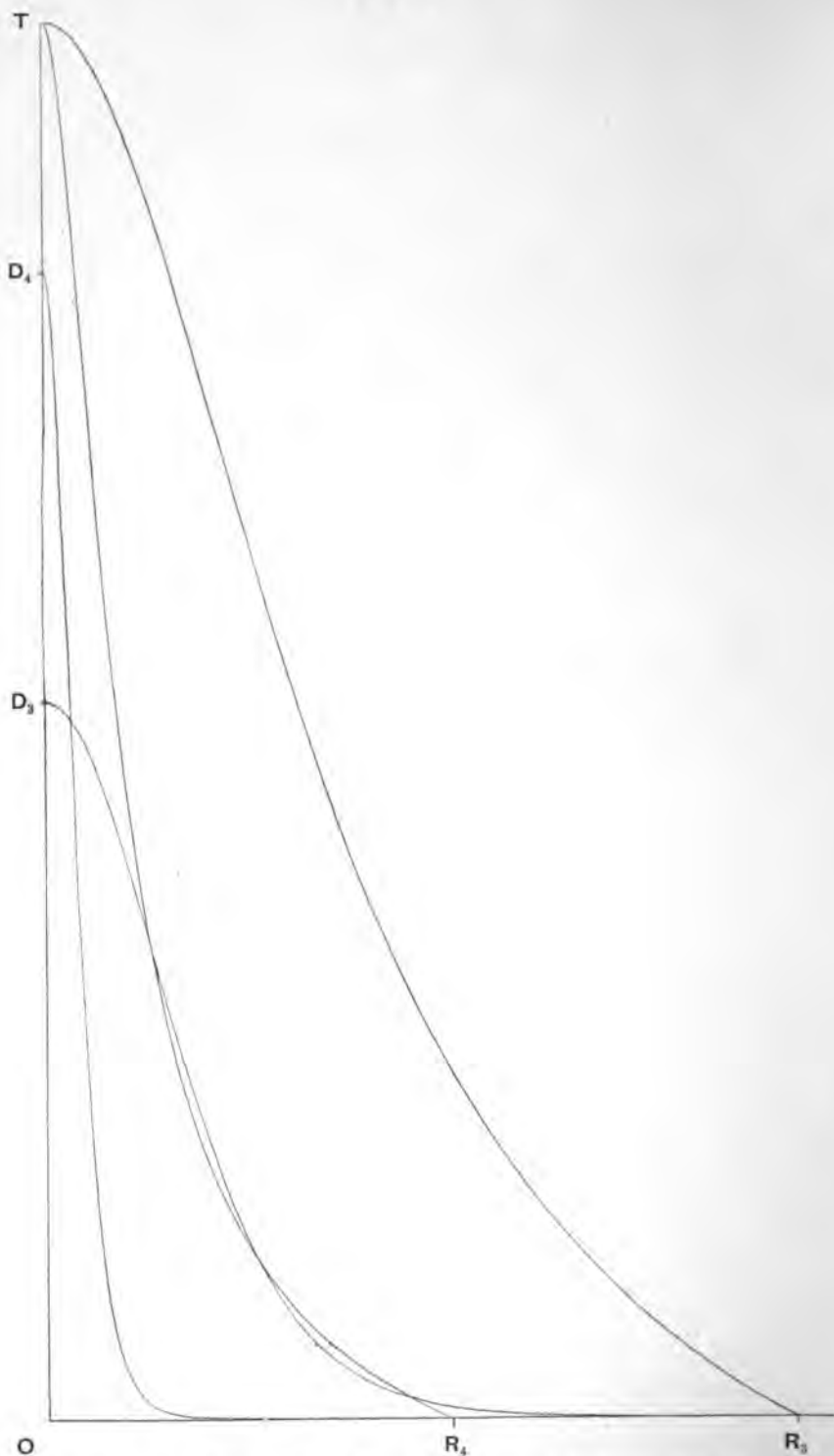
T R_3 is the curve of temperature, and D_3 R_3 is the curve of density, for a gas for which k = 1\frac{1}{2} . T R_4 and D_4 R_4 are corresponding curves for a gas for which k = 1\frac{1}{3} .
